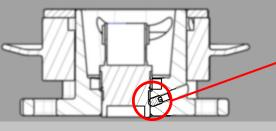
Use Allen Key Size 2 to tighten connector bolt You can use a 2<sup>nd</sup> bolt to secure the first one installed
